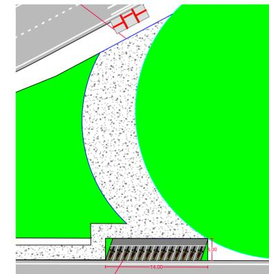
**DETALHE "H" - BARREIRA PRO-MOLDADA EM CONCRETO ARMADO / MURETA DIVISÓRIA DE TRAFEGO**
